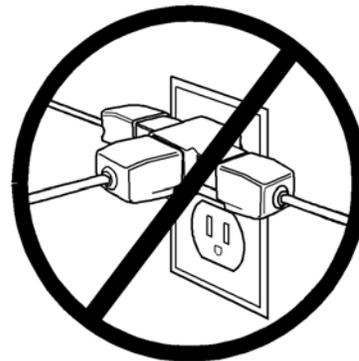
Plug the ventilator into an electrical outlet that is NOT being used to supply electricity to other major appliances. If you need to use the same outlet that is shared by other equipment, make sure the other appliances are NOT being used at the same time.
